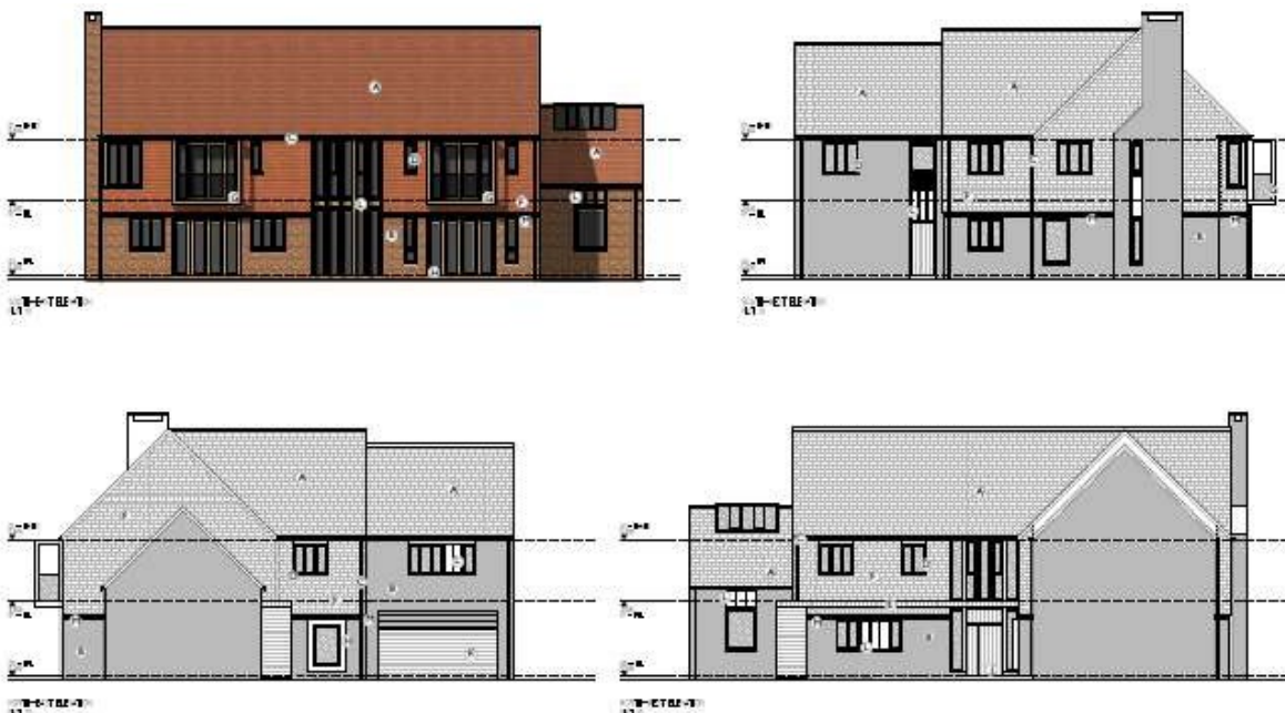
Figure 10: Main house form: Brick and tile hanging with clay plain tiles to roof. Powder coated composite aluminium / timber windows
