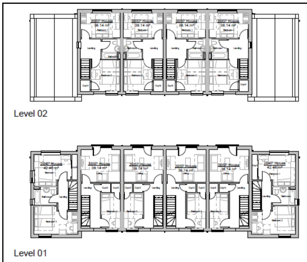
Figure 8 - First and Second Floor Plans - Houses
